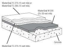
MasterSeal TC 275 (15 wet mils). MasterSeal 941 or equivalent is broadcast then backrolledinto the wet mid coat.
